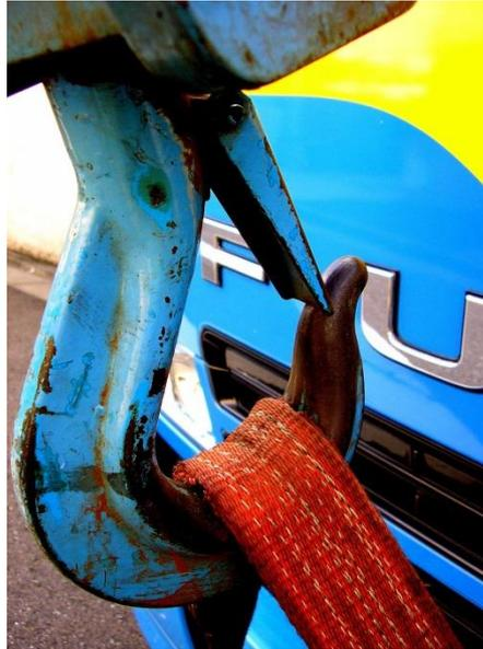
FIGURE 11: CROCHET DE GRUE AVEC LOQUET DE SECURITE FERME. PHOTO DE TANAKAWHO, CC-BY 2.0
