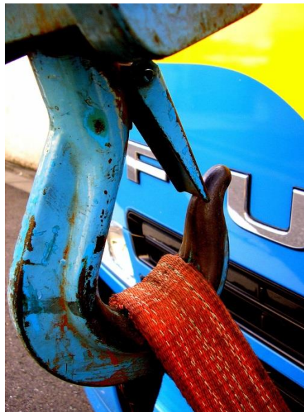
FIGURE 11: CRANE HOOK WITH A SAFETY LATCH CLOSED. PICTURE BY TANAKAWHO, CC BY 2.0
