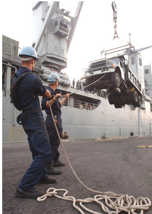
FIGURE 12: WORKERS USING TAG-LINES TO GUIDE THE LOAD DURING A LIFTING OPERATION
